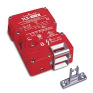
The TLS-GD2 is available in three types. The TLS-1 GD2 and TLS-3 GD2 incorporate a power-to-release function. Two manual release points with security screws allow the locked TLS-GD2 to be released in emergencies. An optional lid-mounted key-release style can also be supplied. The TLS-2 GD2 has a power-to-lock function. Each type of switch has five sets of contacts of various forms and are suitable for use with PLCs.
